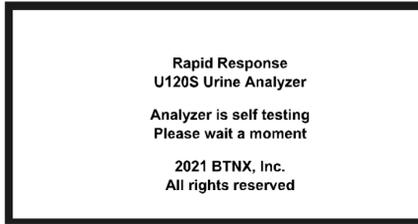
Turn the Power Switch on. If the Self-Test passes, the Initial Screen will be shown.
