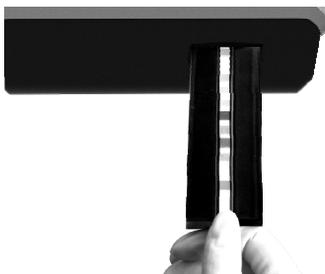
**Note:** In order to avoid contamination of the strip holder and/or the optical sensor, make sure that the strip holder is fully extended and at a standstill before placing or removing a urine strip from the strip holder.
